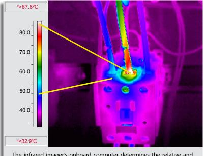
The infrared imager's onboard computer determines the relative and absolute operating temperatures of inspected components.
